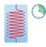
A TWS water heater uses a technique where the hot water from the heat pump is led through a coil in the water to be heated. The water in the heater is also split so that some of the water reaches the correct temperature more quickly. TWS provides more efficient heat transfer and more warm water.
