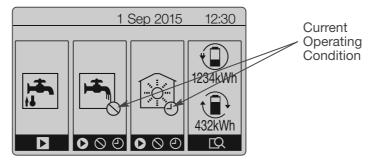
Turning on Priority Hot Water / Hot Water / Heating
