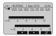
Hours of the day are shown as a bar across the main part of the screen. Where the bar is solid black, heating/DHW (whichever is selected) is allowed.
